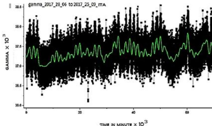
Fig. 5 - Monitoring of gamma radiation between start and time  $70 \times 10^3$  minutes. Green line show smoothed values of 1 day.
