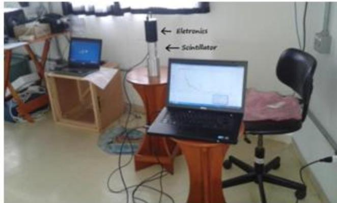
Fig 1. View of scintillator detector with associated electronics and computer laptop on top tower
