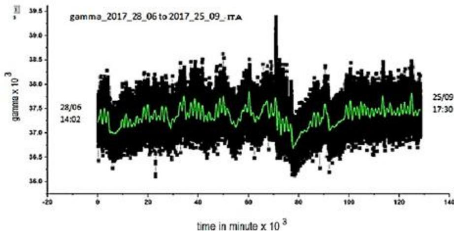
Fig. 4 – Monitoring of gamma radiation in the room at the top of the tower. Green line show smoothed values of 1 day
