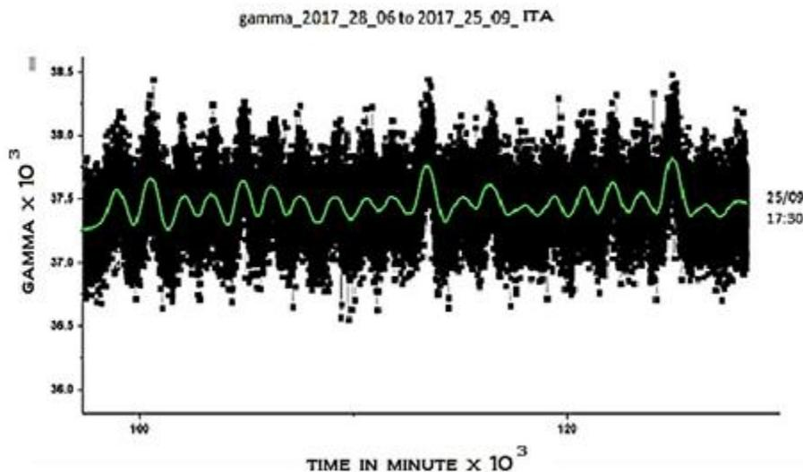
Fig. 12 - Radiation monitoring on dry soil hot by day and cold at night. Green line show smoothed values of 1 day
